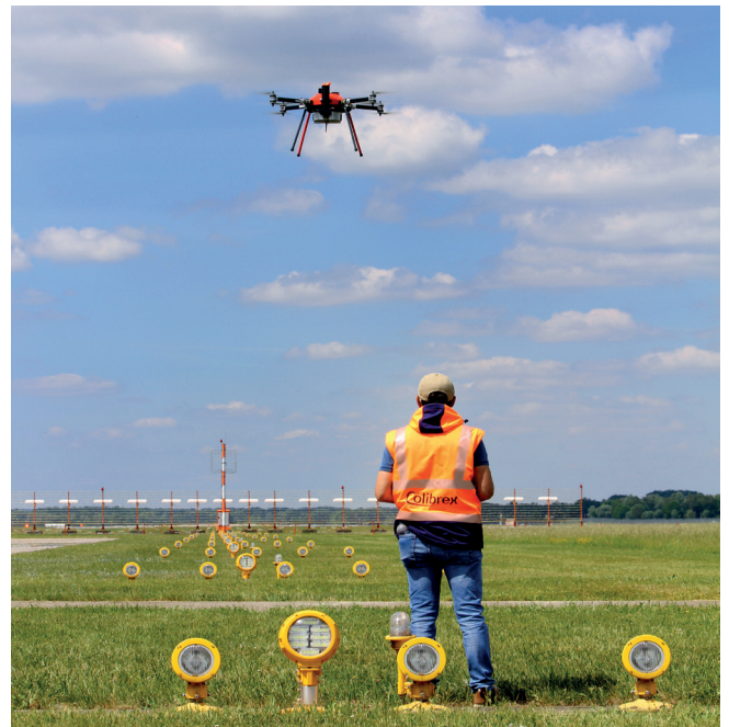
NavAidDrone and pilot in operation
