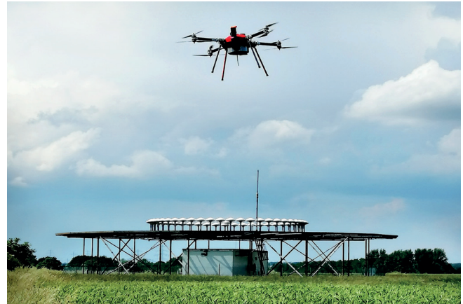
Measurement of VOR signals
